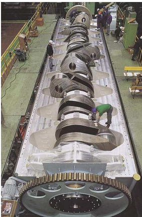
Left: 10 cylinder crank sitting in the block (also known as a "gondola-style" bedplate). Right: A cross section of the RTA96C:
